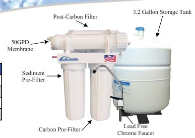
**Reverse Osmosis** is the most effective and economical way to provide your family with high quality drinking water. Reverse Osmosis is a process by which water molecules are forced by your household water pressure through a semi-permeable membrane. Contaminants are rinsed to the drain while your high quality filtered water is stored in a holding tank.
